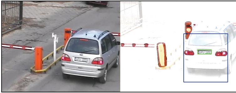
Fig. 12. Example of the license plate detection: original frame from the camera (left) and the processed image (right)
