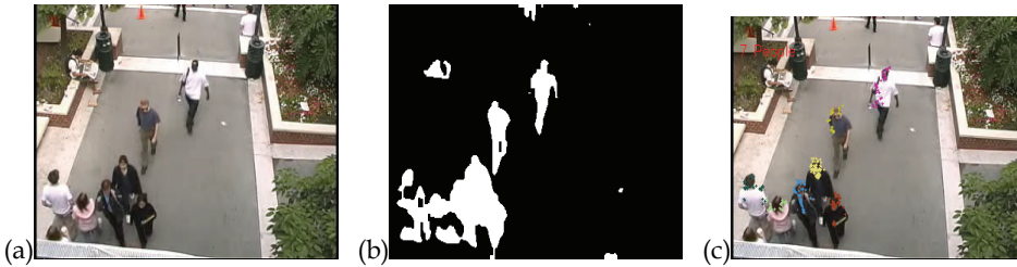
Fig. 9. (a) Original image. (b) The foreground detection with the method of blob-based background subtraction. (c) Target detection and tracking using the point-based feature and each color represents each individual target.
