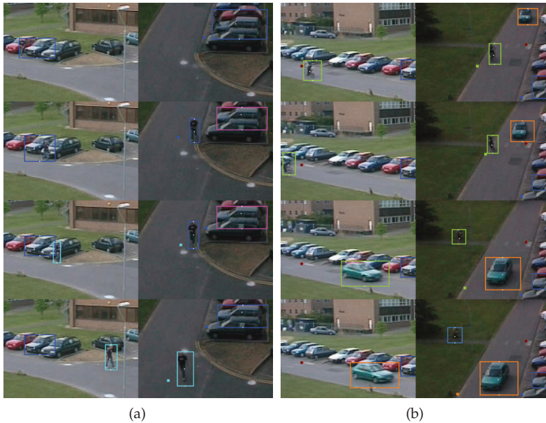
Fig. 13. Fig. 13(a) shows that a man is leaving a car. The system has no prior information about the man in the car and the car is considered as a single object. Due to the warping point deviation, the car in the left view matches the man in the right view. Later, the distance between them is large enough for fixing their pairs. Fig. 13(b) shows that a car enters the left view but it is merged with the bike at the boundary. That mask is considered as same objects before and after the switching during object tracking stage. The error is fixed at the SCL stage.
