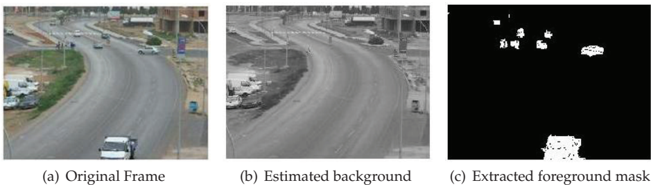
Fig. 7. Background / Foreground separation using group based histogram method
