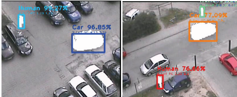
Fig. 8. Examples of classification results obtained using the shape recogniser, with temporal probability denoted
