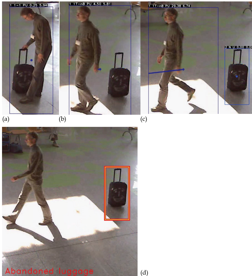
Fig. 14. An example of abandoned luggage detection: (a) initial state, (b) detected left luggage, (c) detected person away from luggage, (d) detected luggage still unattended, high-level event 'abandoned luggage' detected, visual alert
