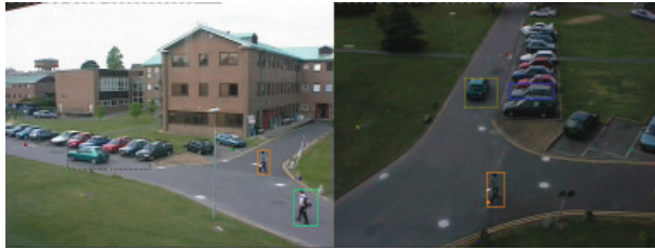
Fig. 12. Spatial consistency labeling result. The merged object in left view contains green, red, and blue tag which represents the driver, the green car, and the dark blue car in turn. If an object in the left view is a single object, its transformed ground point is shown in the right view.
