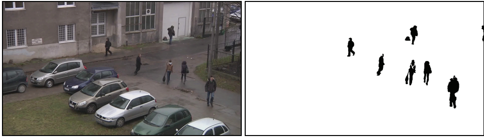
Fig. 3. Example results of moving object detection: original video frame (left) and binary mask denoting moving objects (right)
