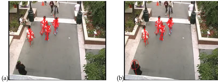
Fig. 13. Grouping of new points. (a) Green points are the new generated points that are distant from other existed red clusters. (b) The result of clustering.
